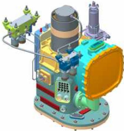
MOMA performs gas chromatograph pyrolysis injections with known gases.
