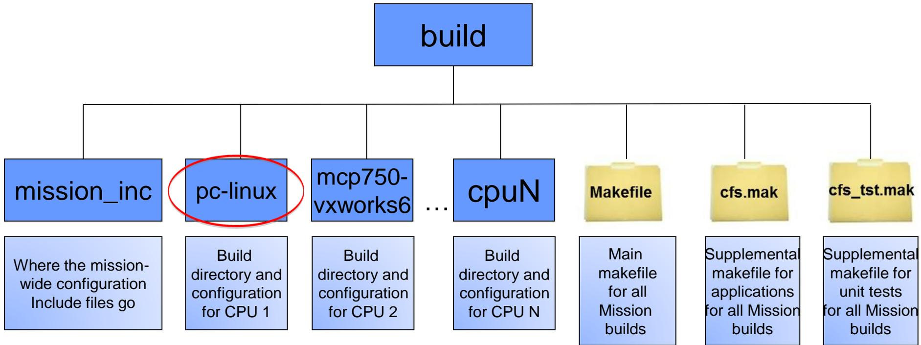
The “build” directory is where the cFS ( cFE Core + cFS Apps ) is built for a mission. This directory contains all configured mission and platform configuration files.
