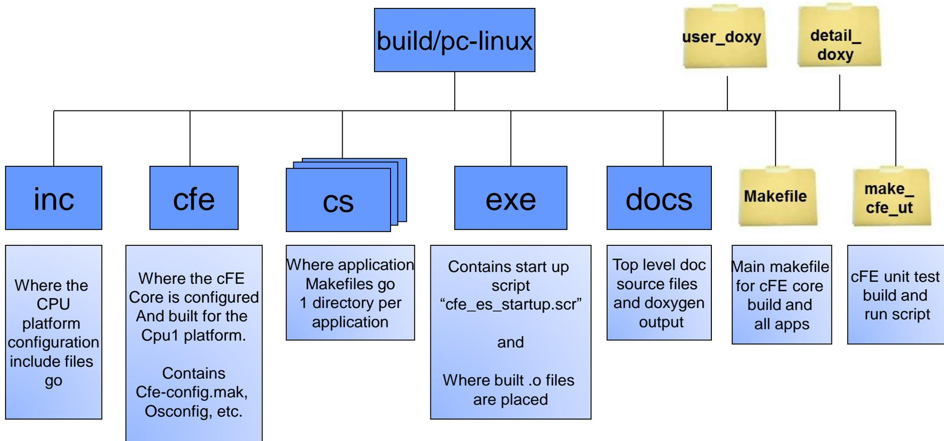
Each Platform ( CPU ) directory can have a custom cFE core configuration which is built for a specific architecture, platform, and operating system. It can have a unique mix of cFS applications.
