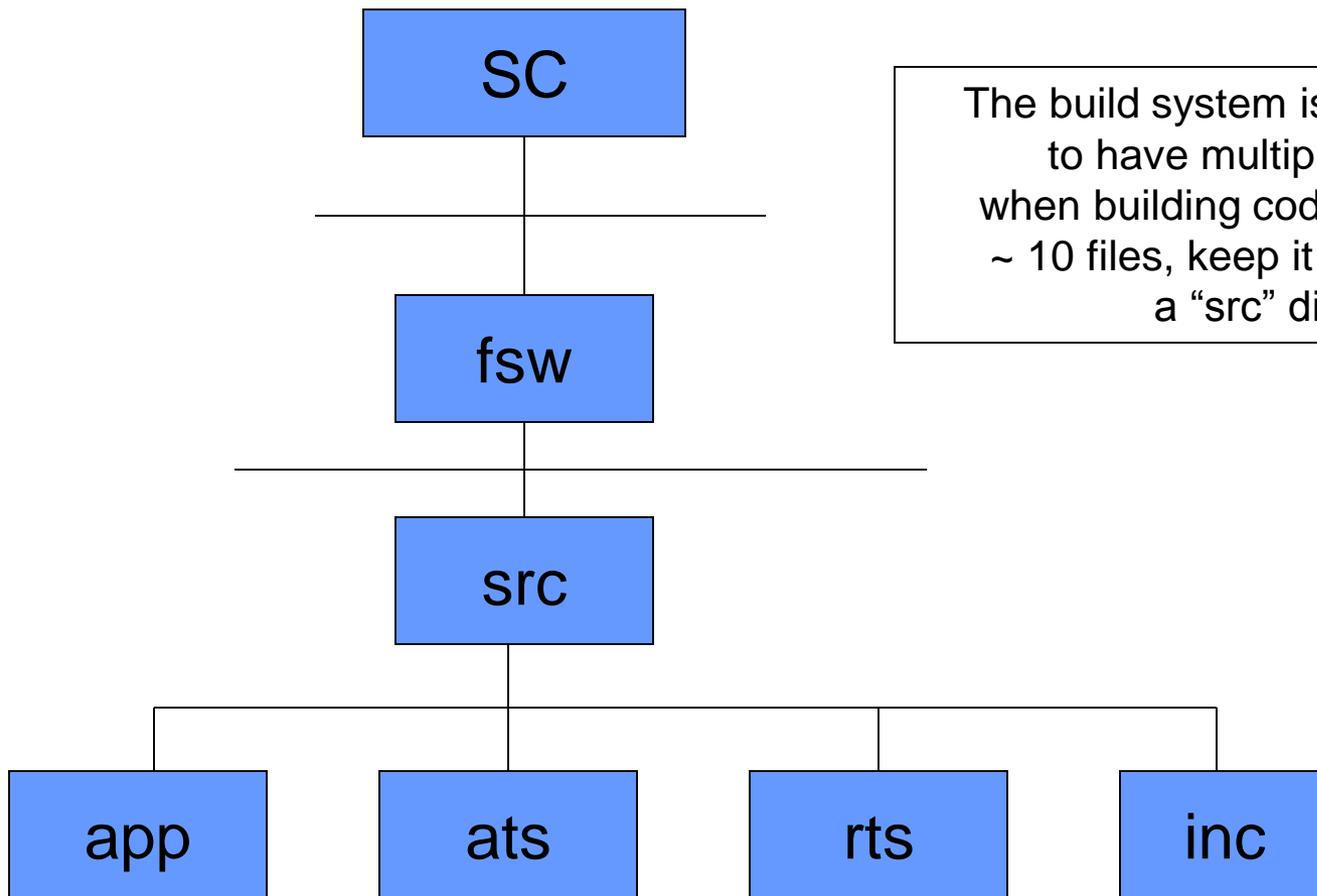
The build system is flexible enough to have multiple directories when building code. For apps with ~ 10 files, keep it simple with just a “src” directory
