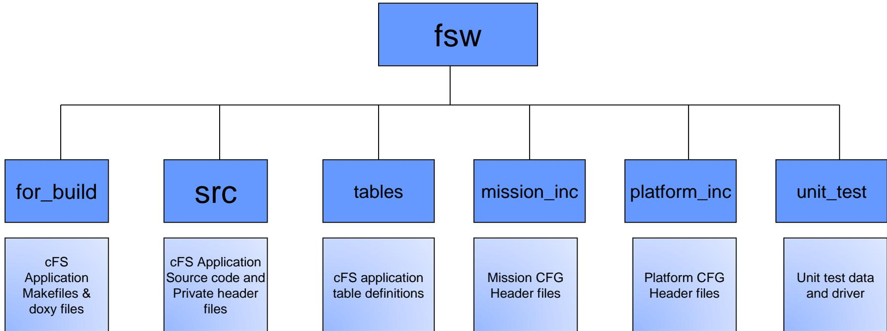
The “fsw” directory is where all of the software for the cFS Application is stored. The “src” directory includes all private header files and C source files. The remaining directories have public and configuration header files to be installed in the cFS Mission Directory Structure.
