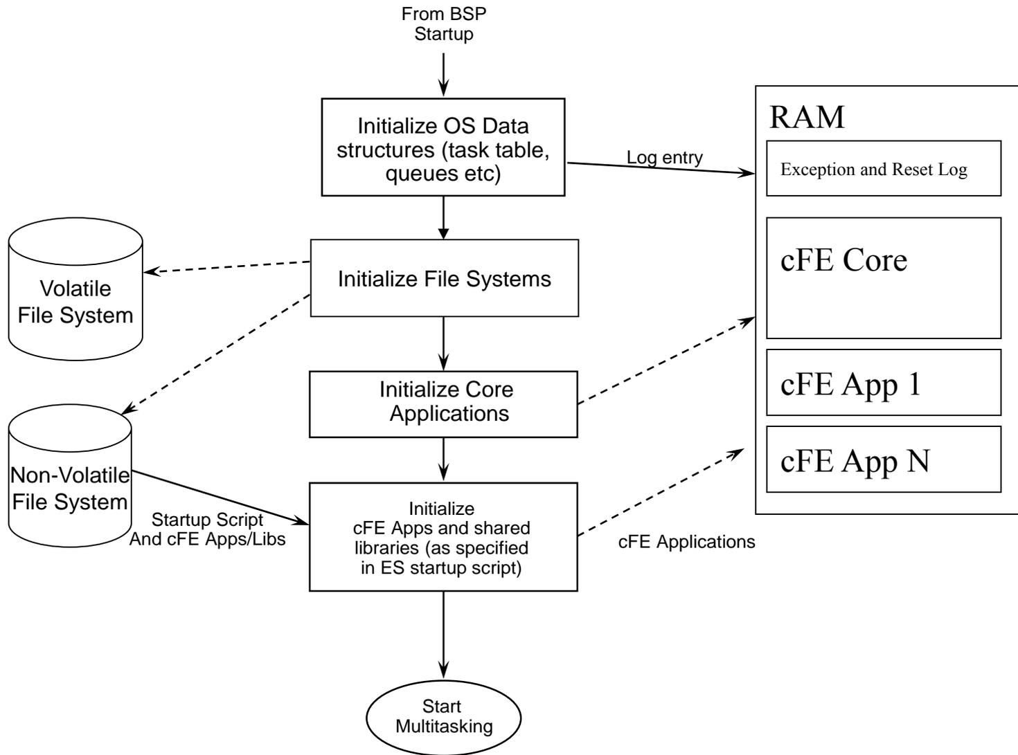
The cFE core is started as one unit. The cFE Core is linked with the RTOS and support libraries and loaded into system EEPROM as a static executable.
