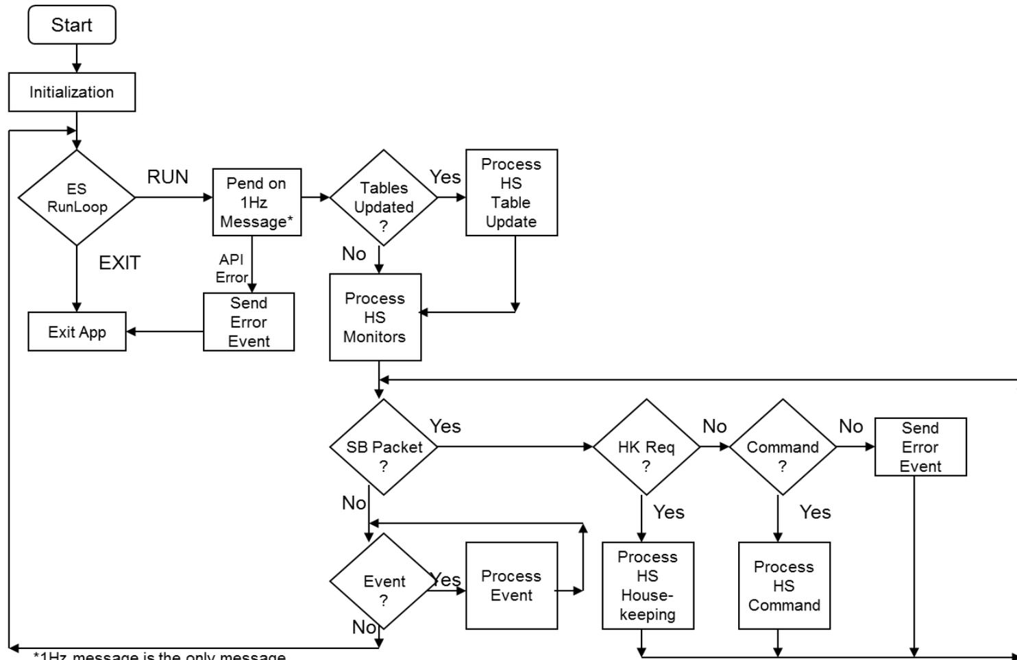
\*1Hz message is the only message that shows up on that pipe, and is a pend with timeout.
